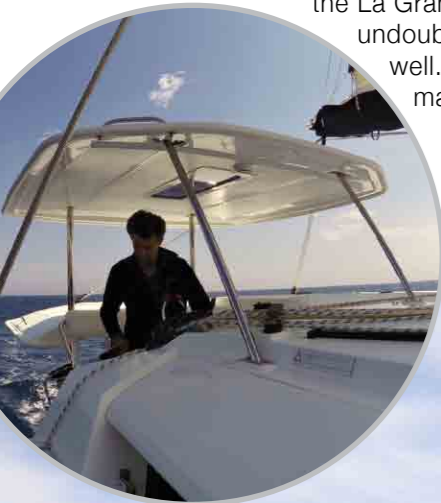
All controls are centralised so ideal for short-handed sailing and the fibreglass bimini can have a plastic front for weather protection. Photo Kevin Green
