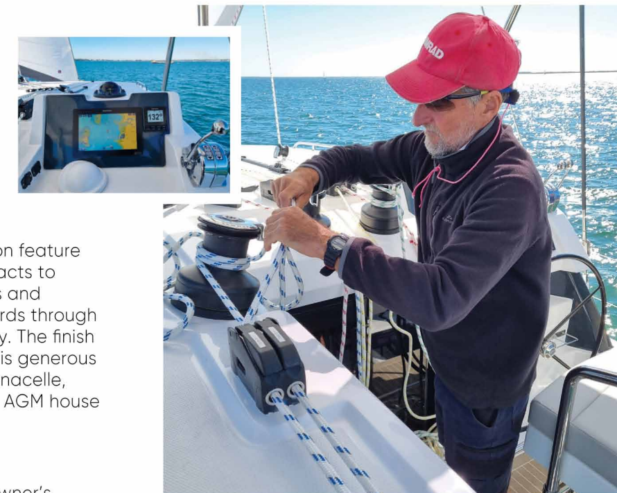
ABOVE: All sail controls run to the steering console which has enough space for trimmer and a steerer. Image Kevin Green
