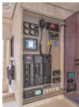
The electrical panel includes a Raymarine A65 control screen for the menu driven domestic controls. Image Leopard Catamarans
