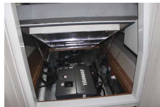
ABOVE LEFT: The aft beds are electrically lifted to reveal the shaft driven Yanmars and there's separate access to the transom bulkheads where generators and air conditioners are located. Image Kevin Green
